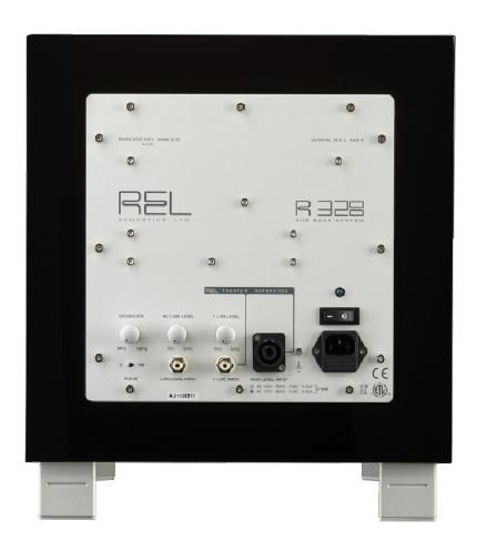
Also on the rear panel are a smoothly rotating output-level knob, a knob for setting the crossover frequency that operates from 30 to 120Hz in small clicks, and a phase switch: 0° or 180°. Two last things to note: It's a shame that the R-328 will be tucked into a corner; its hand-rubbed, gloss-black finish is impeccable.
